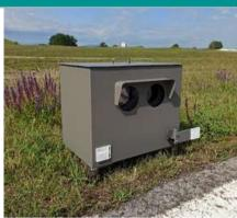
The RSD6000 can be quickly deployed on the roadside in protective boxes, for quick and easy deployment. This configuration allows the RSD6000 to be easily transported and placed at a specific site without any prior preparation.
