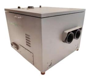
The above measurements lead to the automatic reporting of the pollutant concentrations relative to CO2: CO/CO2, NO/CO2, NO2/CO2, HC/CO2 and NH3/CO2. It also provides the Smoke Factor (SF), to evaluate the vehicle's exhaust particulate matter emissions.
