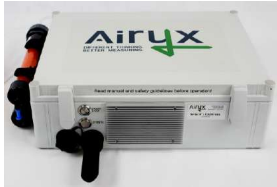
Figure 3: Mobile ICAD NO x instrument of Airyx GmbH used for Plume chasing. The instrument fits in the easily in any car boot.
