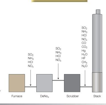
The OPSIS monitoring system is an effective tool for controlling the different emissions and process control spots in a waste incinerator
