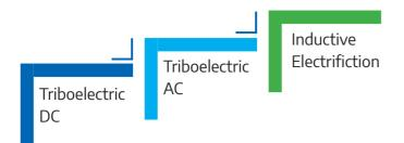
The measurement of Sintrol dust monitors is based on particles interacting with an isolated probe mounted into a duct or stack. When moving particles pass nearby or hit the probe, a signal is induced. This signal is then processed through a series of Sintrol's advanced algorithms to filter out the noise and provides the most accurate dust measurement.
