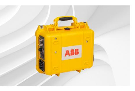
Sensitive, fast and compact analyzers for measurement of CH₄, CO₂ and H₂O
