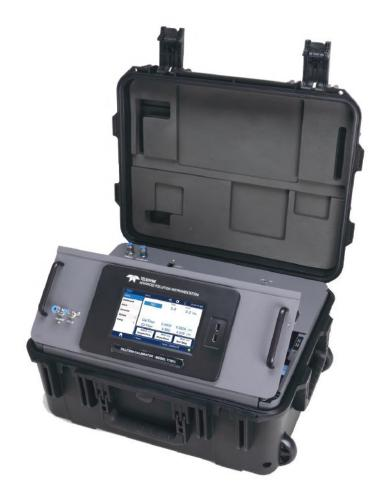
A portable, microprocessor based calibrator for precision gas analyzers, the Model T750U combines highly accurate mass flow controllers and compressed sources of standard gases to provide multipoint span and zero calibrations. The T750U includes two operating modes: a high range with similar performance to the Model T750 instrument with ozone generator, and a low range which includes a "fractional mode" for producing accurate and stable O<sub>3</sub> and NO<sub>2</sub> levels down to 3 ppb.
