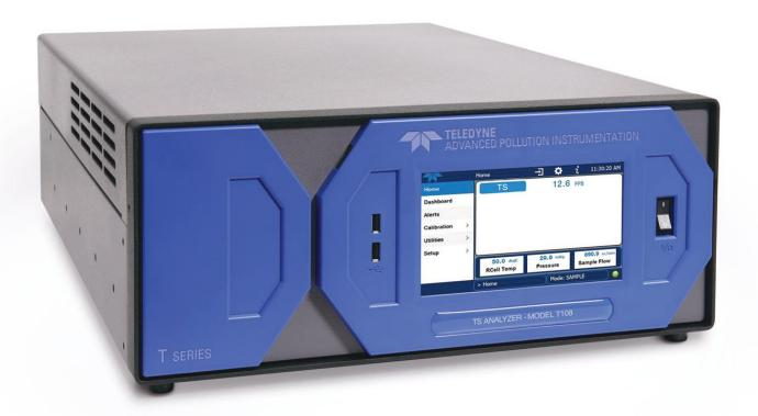
The Model T108 Total Sulfur analyzer is designed to measure mixed sulfur impurities, collectively referred to as Total Sulfides, in air or carbon dioxide gas. The model T108 consists of a modified Model T100 SO<sub>2</sub> analyzer with special software and a Model 501TS SO<sub>2</sub> high temperature thermal oxidizer.
