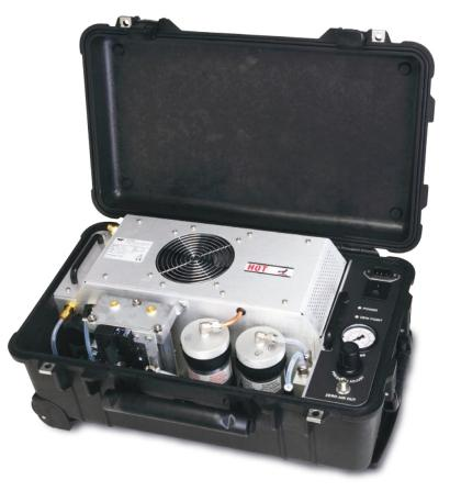
A portable, fully self-contained source of high purity zero air for dilution calibrators, the Model 751H is ideal for use with sensitive analyzers in ambient background and trace level applications.
