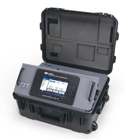
A portable, microprocessor based calibrator for precision gas analyzers, the Model T750 combines highly accurate mass flow controllers and compressed sources of standard gases to provide multipoint span and zero calibrations. UV ozone generator, photometer, and gas phase titration (GPT) chamber options are also available for the T750 for stable and accurate O<sub>3</sub> and NO<sub>2</sub> production.
