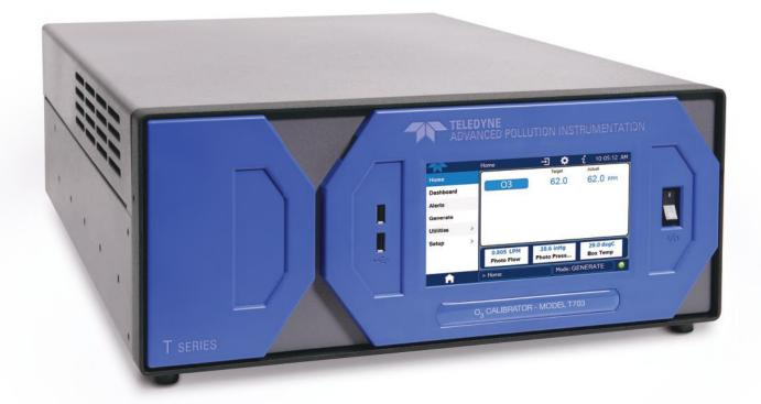
The Model T703 Photometric  $O_3$  calibrator combines an ozone generating device and photometer to provide a specified ozone concentration by volume for precision gas analyzers.
