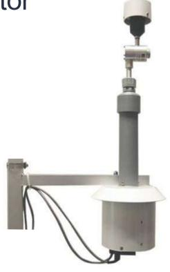
The NPM 3 is calibrated using 0.6µm NIST traceable polyspheres. These provide a critical and consistent baseline calibration. To correlate this calibration to real-world, non-spherical particulates, a Calibration Factor (K-Factor) is established by means of comparison to a collocated, trusted, and proven reference source (i.e., a BAM 1020) to ensure both accuracy and correlation.
