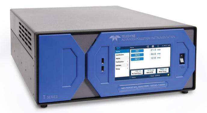
The Model T200M Mid-Range NO /  $NO_2$  /NO $_X$  analyzer uses the proven chemiluminescence detection principle and advanced electronics to allow accurate, dependable, continuous measurements for mid-level stack gas monitoring and other applications. The T200M may be fitted with an optional, internal paramagnetic  $O_2$  sensor or an infrared absorption  $CO_2$  sensor, reducing integration and operating costs significantly.
