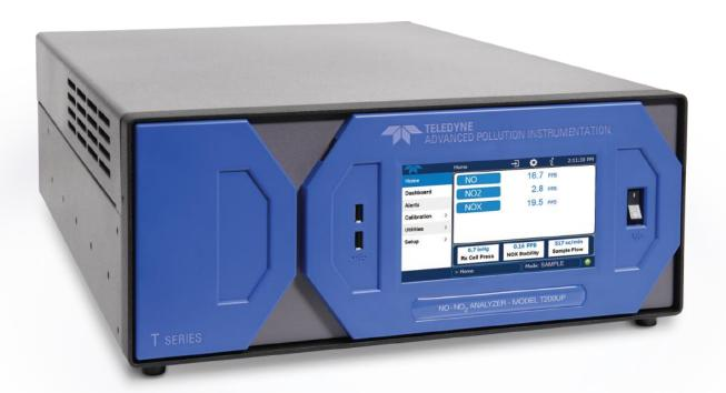
The Model T200UP provides Trace Level measurements of NO,  $NO_x$  and  $NO_2$  using our proven T200U  $NO_x$  analyzer combined with a patented high efficiency Blue Light Converter (BLC), also known as photolytic converter. The BLC provides a very specific conversion of  $NO_2$  with conversion efficiency similar to molybdenum but without the same interferences.\* The T200UP provides ultra-sensitive performance and is ideal for ambient and roadside monitoring.
