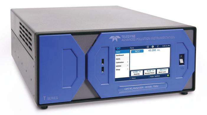
The Model T500U NO<sub>2</sub> analyzer is a significant advancement in the direct measurement of NO<sub>2</sub> using a Cavity Attenuated Phase Shift (CAPS) spectroscopy technique to provide highly accurate, real-time, continuous, and direct readings. The T500U offers a cost effective and low maintenance instrument package ideal for ambient and roadside monitoring.
