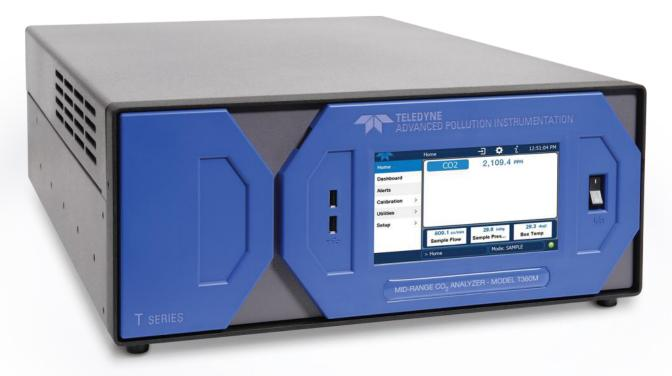
Using a gas filter correlation wheel, the Model T360M Mid-Range  $CO_2$  Analyzer measures carbon dioxide by comparing infrared energy absorbed by a sample to that absorbed by a reference gas according to the Beer-Lambert law. This design produces excellent zero and span stability and high signal to noise ratio, allowing excellent performance over a wide concentration range, making this instrument an ideal choice for  $CO_2$  reporting requirements associated with dilution CEMS.
